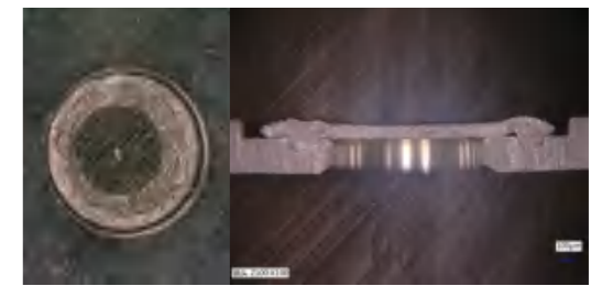
密封钉焊接 Sealing nail welding
