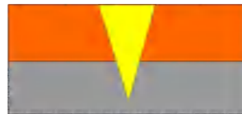
长脉冲激光熔池 呈V字形, 易击穿, 强度低 Long pulse laser bath V-shaped, easy to break down, low strength
